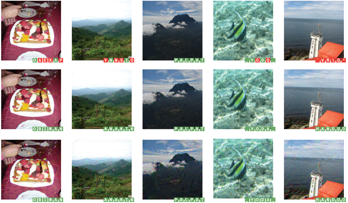
Fig. 5: Watermarked images from the INRIA Holidays dataset resized to 128 \times 128 . The watermark is added with our multi-bit watermarking method with a payload of 30 bits and with different values for the target PSNR: 52dB (top row), 40dB (middle row), 32dB (bottom row). We use a 5-bits character encoding to encode and decode one message per image, and show the decoded messages for each image (without any transformation applied to the image). The higher the PSNR, the higher the decoding errors, and the less robust the decoding is to transformations.
